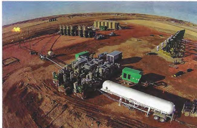
**Fig. 3.** The units manage the varying hydrocarbon flow and chemistry changes inherent to producing wells. They also compress the associated flare gas to 150 psi and lower the temperature to -35°F (normal frost build-up shown bottom center).
