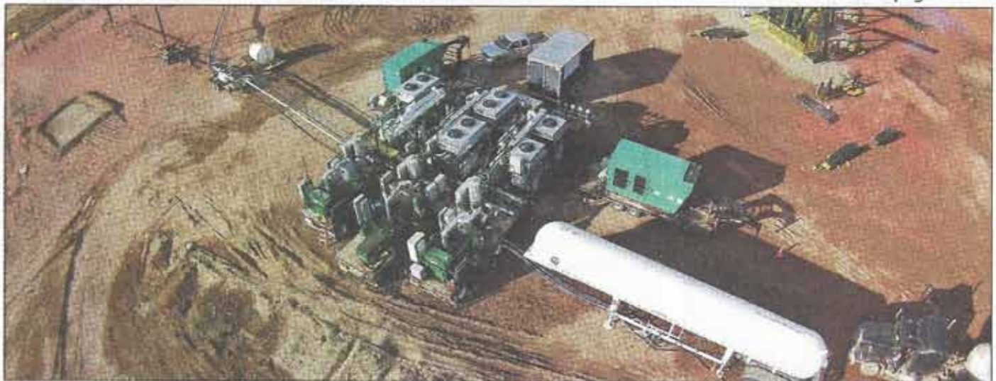
These three GTUIT field natural gas stripping units are on a Hess Corp. well pad in McKenzie County. The Billings, MT service company uses these mobile units on remote locations to strip and freeze NGLs as an alternative to flaring. (GTUIT Photo)
